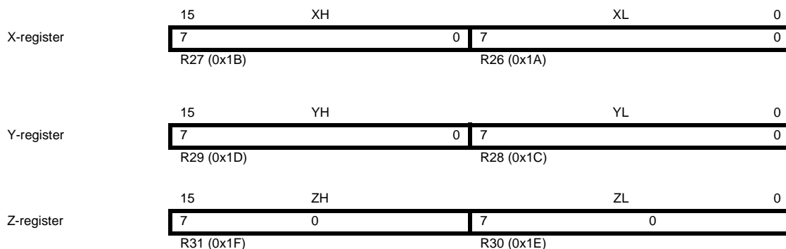
Figure 4-3. The X-, Y-, and Z-registers
