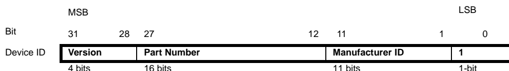
Figure 26-1. The Format of the Device Identification Register
