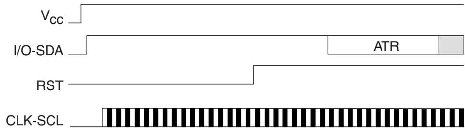
After a successful ATR, the Protocol and Parameter Selection (PPS) protocol, as defined by ISO 7816-3, may be used to negotiate the communications speed with CryptoMemory devices 32 Kbits and larger. CryptoMemory supports D values of 1, 2, 4, 8, 12, and 16 for an F value of 372. Also supported are D values of 8 and 16 for F = 512. This allows selection of 8 communications speeds ranging from 9600 baud to 153,600 baud.
